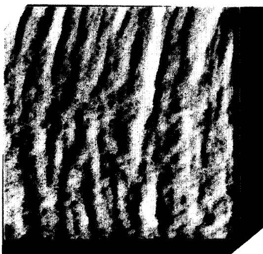
Figure 2 Morphological image of Fibre A observed by AFM, 500 \times 500 \text{ nm}^2 : (a) 'constant height mode', 2D presentation; (b) 'constant force mode', 3D presentation
